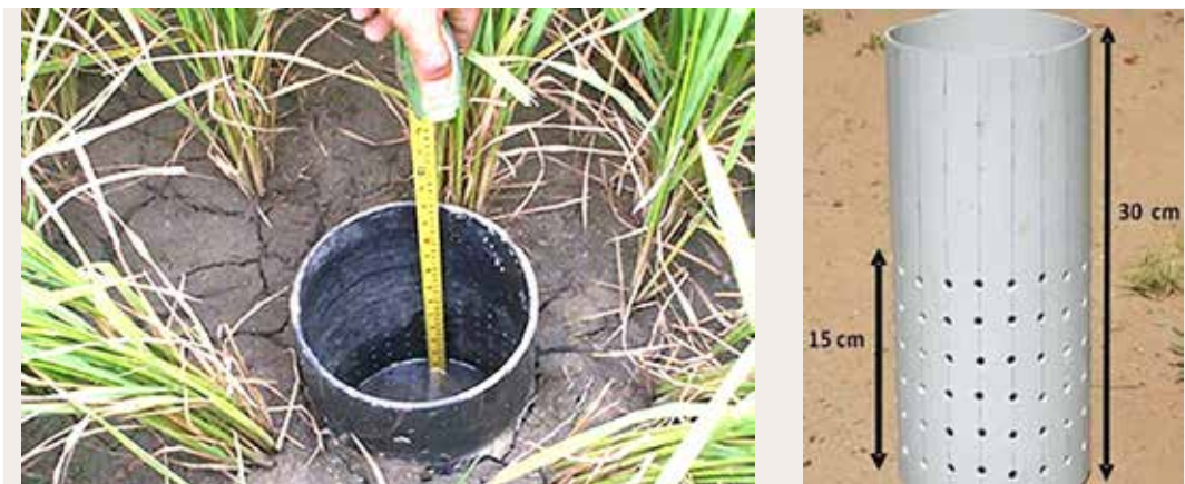
Figure 20: Alternate wetting and drying (AWD) technique for water management
